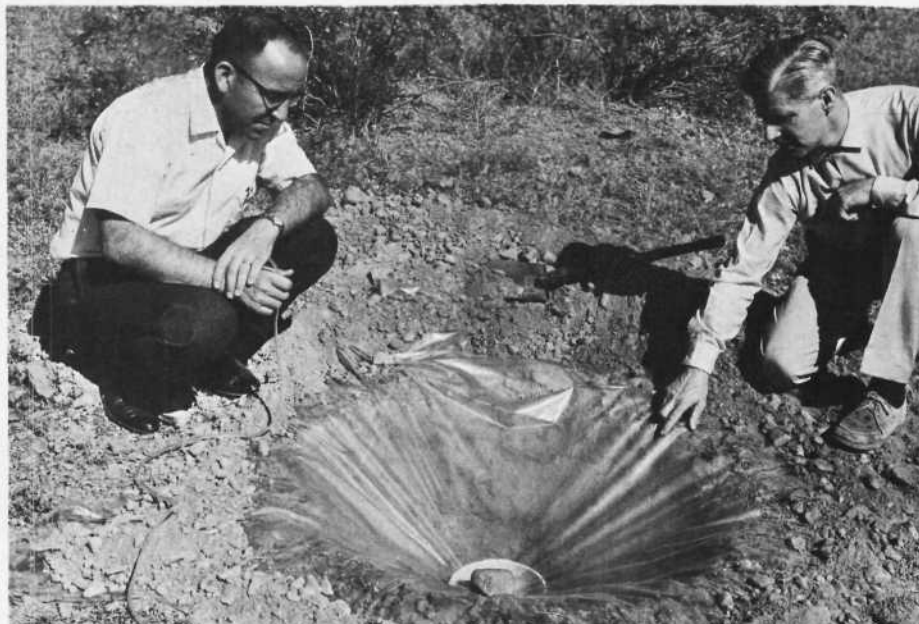
Chop up the bisnaga, put it in hole with container. Cover hole with Tedlar plastic and place weight in center above container.
