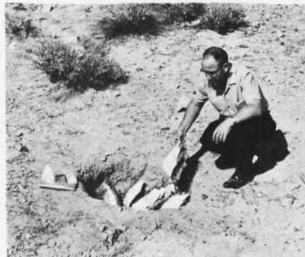
Chop up the bisnaga, put it in hole with container. Cover hole with Tedlar plastic and place weight in center above container.
