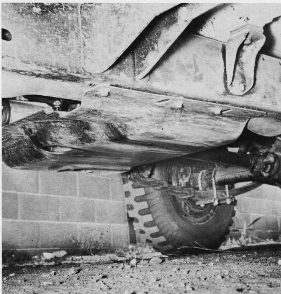
RUGGED STEEL BELLY-PAN PROTECTS UNDERSIDE OF LAND CRUISER. THIS IS EXCELLENT SAFETY FEATURE IN ROCKY TERRAIN.
