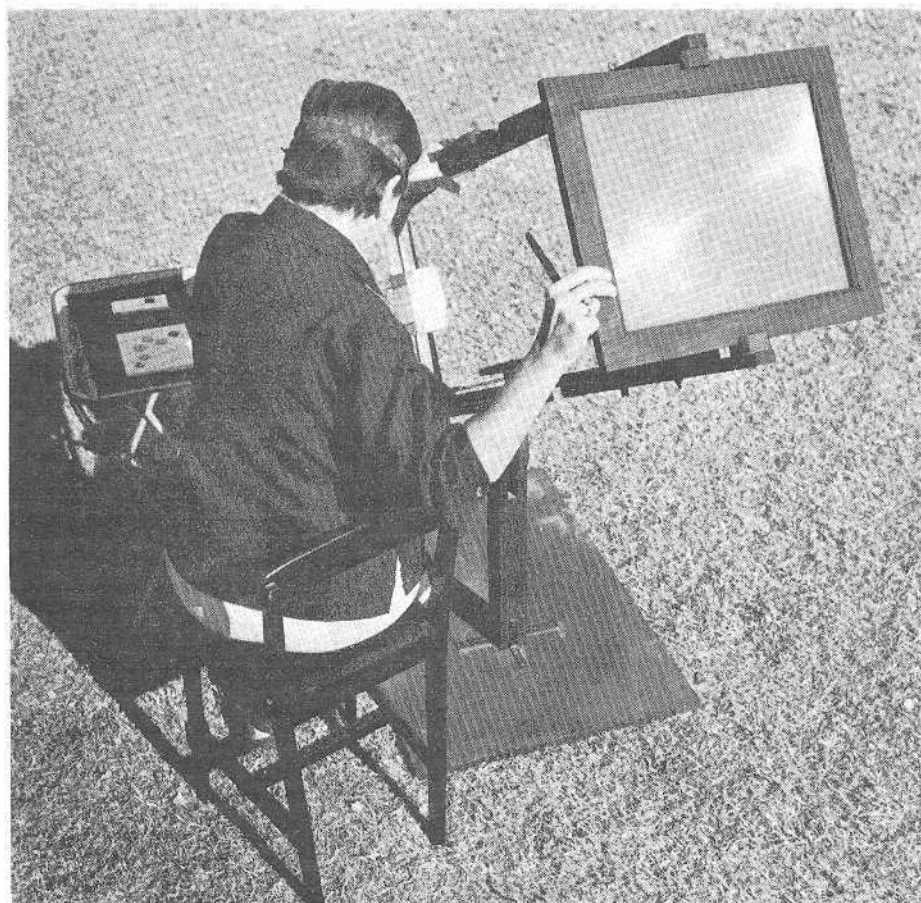
Operator adjusting the plastic fresnel lens to control the focal point of sunlight on the ceramic brick oven.
