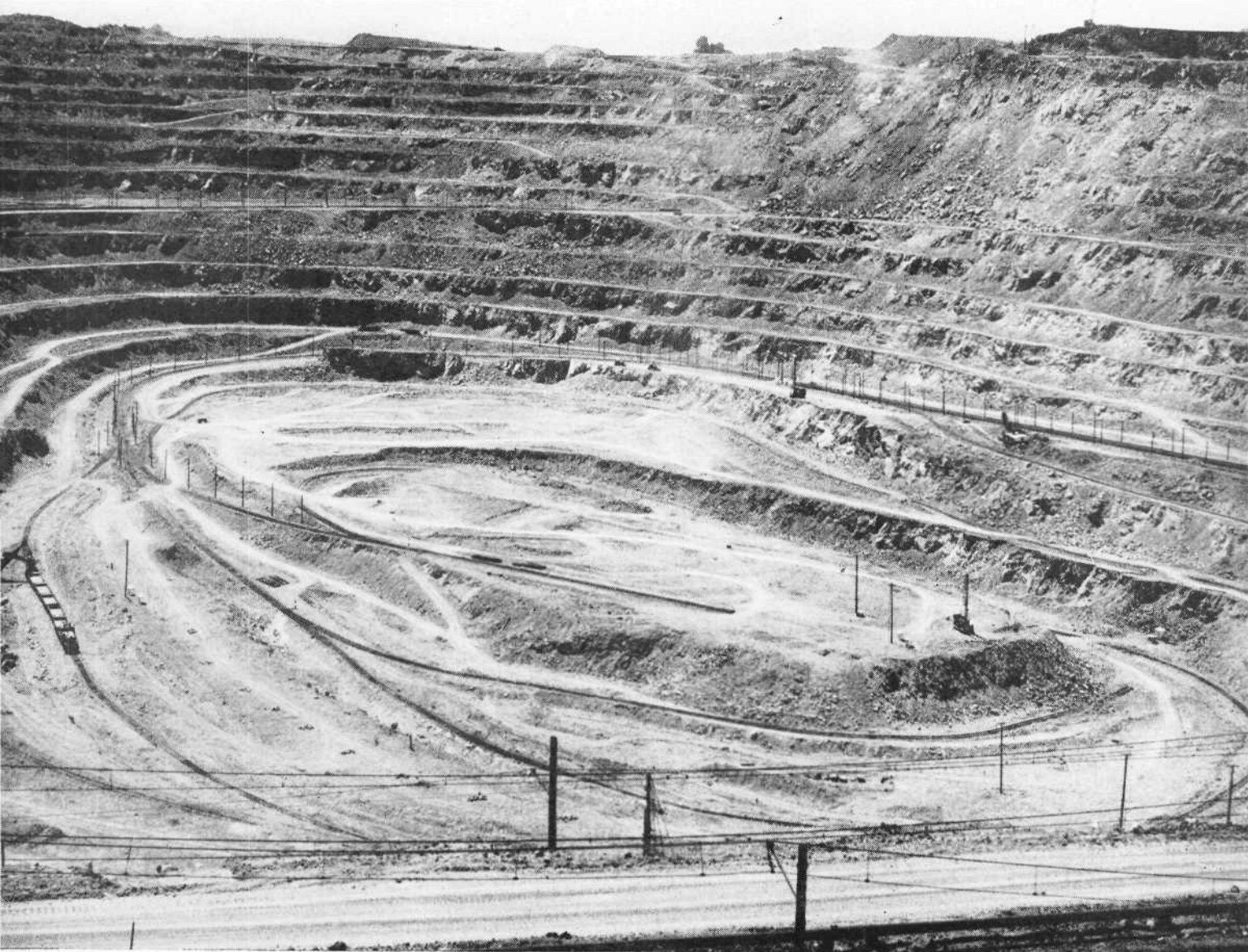
Giant electric shovels resemble toys in the 550-foot deep open copper pit which has made Ajo the nation's third-ranking copper producer. Open pit method began in 1917.
