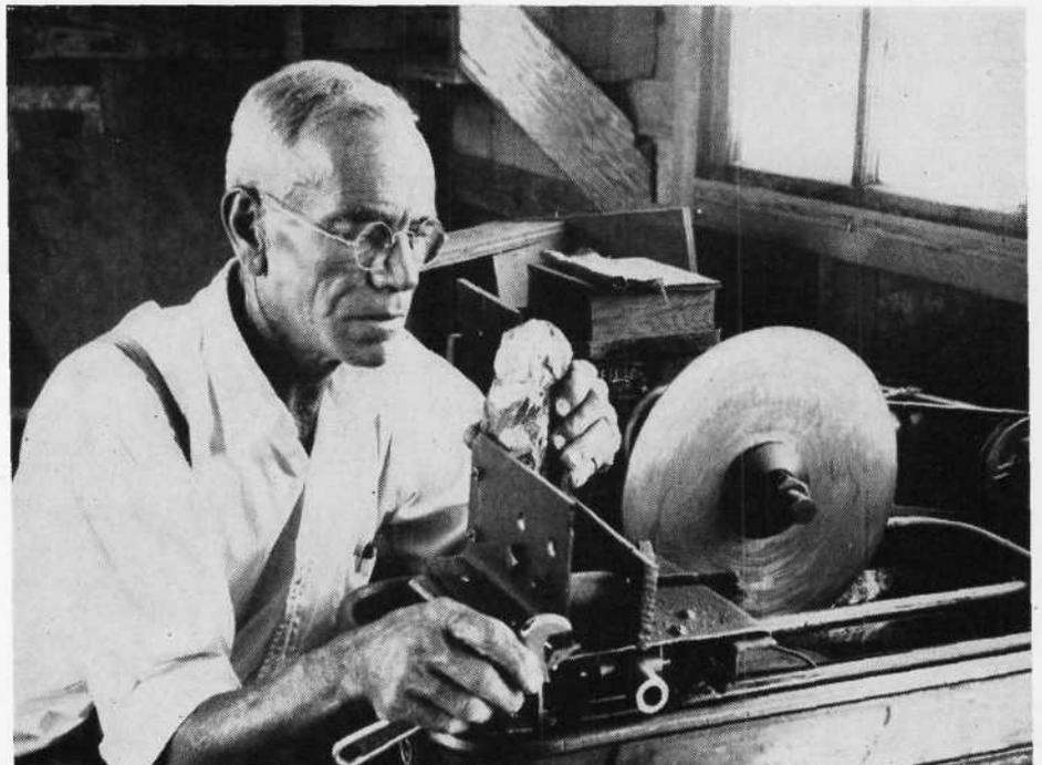
*Herbert Kibler with the rock-saw he built from the bed of a child's wagon and odds and ends from junked automobiles. And it works!*
