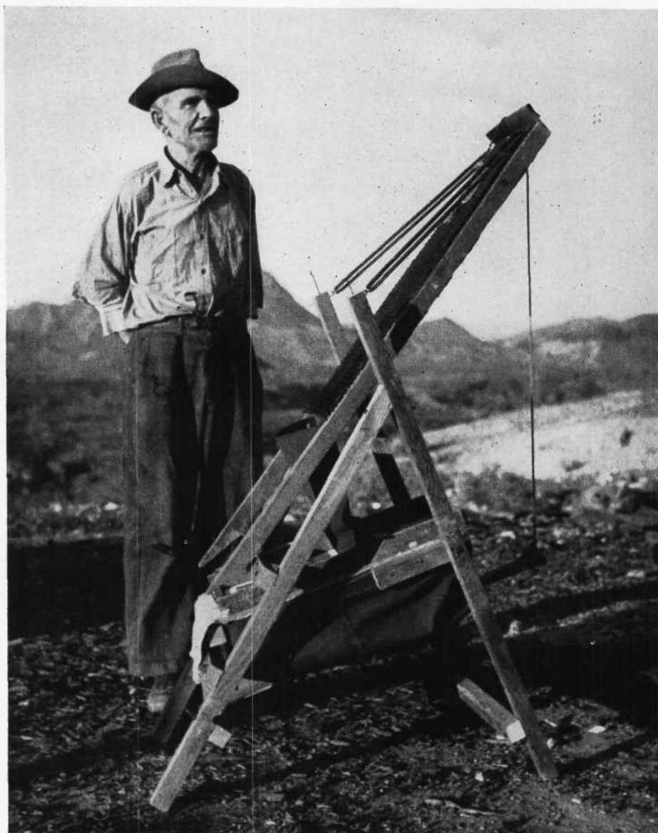
Charlie Johns, prospector in the Mesquite Diggings area near where the lost Harpending silver dike is located. This dry washer was invented by Dan Saylor, also of Mesquite Diggings.
