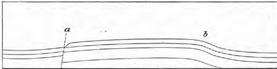
FIG. 3.—Section across the Kaibab. The vertical scale is double the horizontal. a , West Kaibab fault. b , East Kaibab monocline. Length of section about 32 miles.
